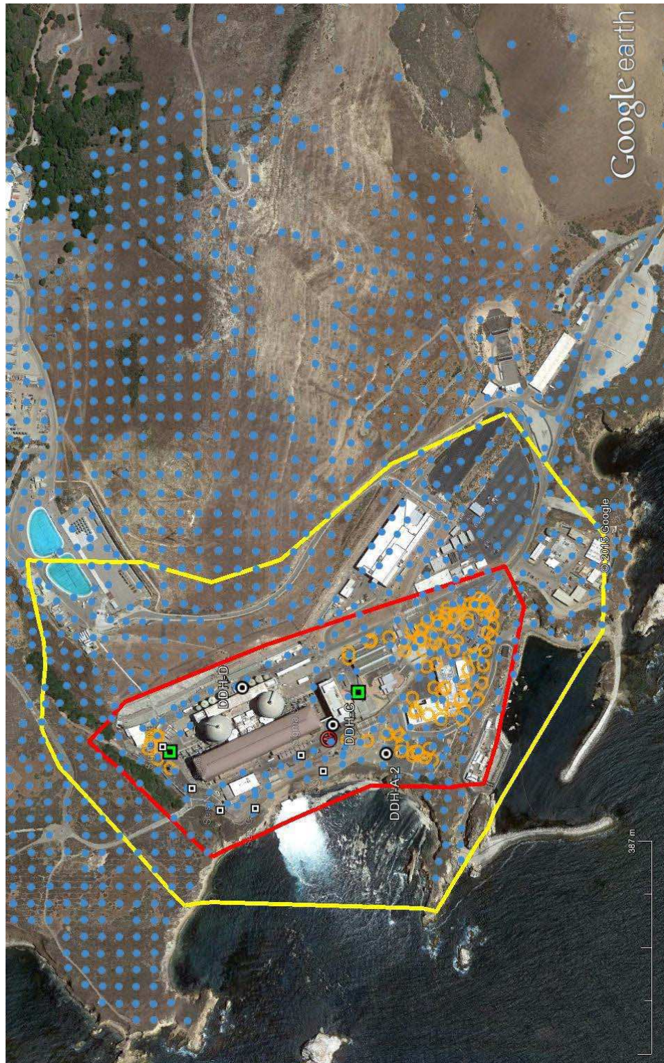
DCPP FOUNDATION AREA ZLAND NODES (BLUE CIRCLES) AND NODE GROUP CENTROIDS (ORANGE CIRCLES) (ZLAND NODES WERE USED INSIDE THE RED POLYGON AND VIBROSEIS SOURCES WHERE USED WITH THE YELLOW POLYGON) Update of the 3-D Velocity Model for the DCP Foundation Area San Luis Obispo, California
